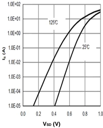
Figure 7: Body-Diode Characteristics
