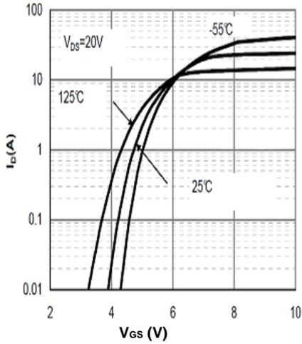
Figure 3: Transfer Characteristics
