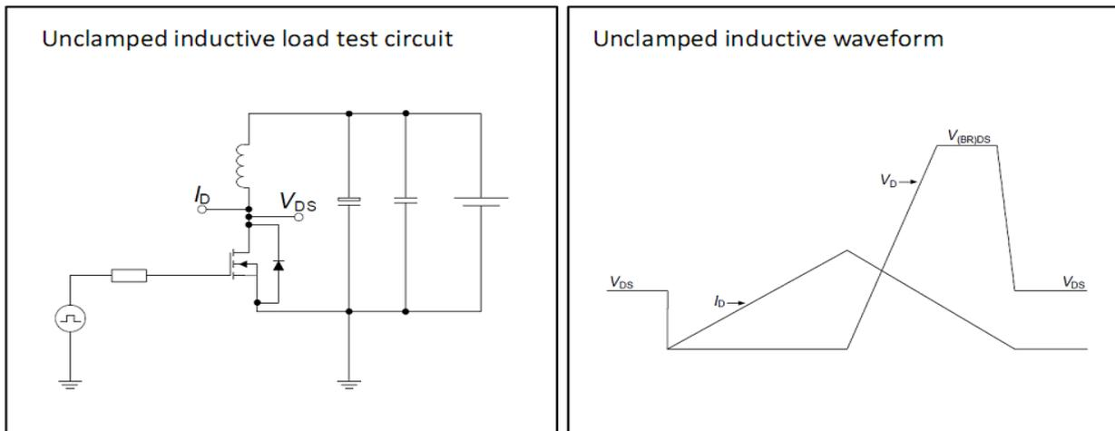
Test circuit and waveform for diode characteristics
