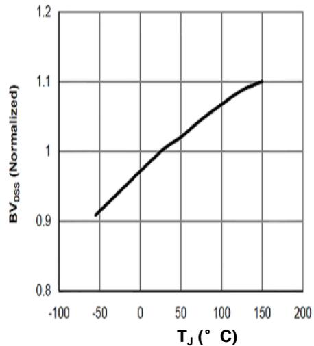
Figure 6: Break Down vs. Junction Temperature
