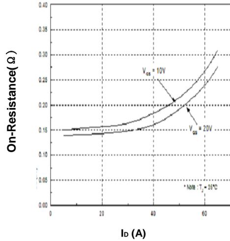
Figure 4: On-Resistance vs. Drain Current ( $I_b$ )
